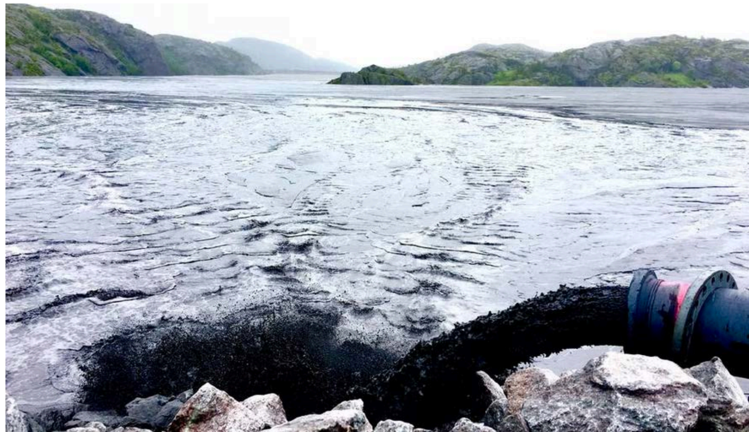
TSF land fill from the Titania mine in Sokndal, Norway. Without watering, dry tailings from the Titania TSF would create significant dust pollution. It's necessary to mitigate this substantial water application performed through manual watering using tractors and sprinkler systems. Photo: Mathias Oppedal.
